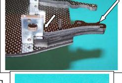
B9) Turn the chassis over and install the nose piece with the post to the top of the chassis. Use the four 5/8" Cap Head screws (XF 6003).
