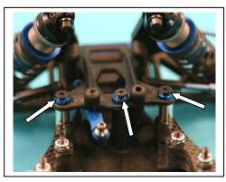
B12) Turn the car over and use the flat head screws you saved to install the bulkhead to the nose piece. When everything is right, tighten the two bottom screws and the three on top from B11,
