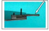
B4) Using a 3/8" Flat Head screw (XF 6022) from Bag B (arrow) and the 5/8" flat head, install a Top Deck Support (XF 1400). If you are using thread lock, a drop now in the bottom holes of the support.
