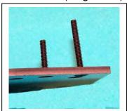
B2) Place a Nose Bridge Spacer (XF 1534) over the two bolts.
