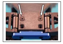
B13) Use the saved flat head screws to put the bumper on.
