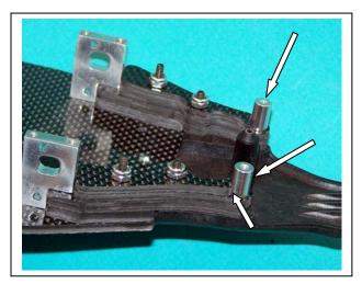
B11) Place the complete front suspension and steering on the X – 6 Cubed just as it was on the B 4.2. Secure the top plate (AE 9566) with the three screws and countersunk washers that were on the B 4.2. Drivers using thread lock should put a drop in the stand-offs. Finger tight for now. Make sure the top plate is snug with the nose piece.
